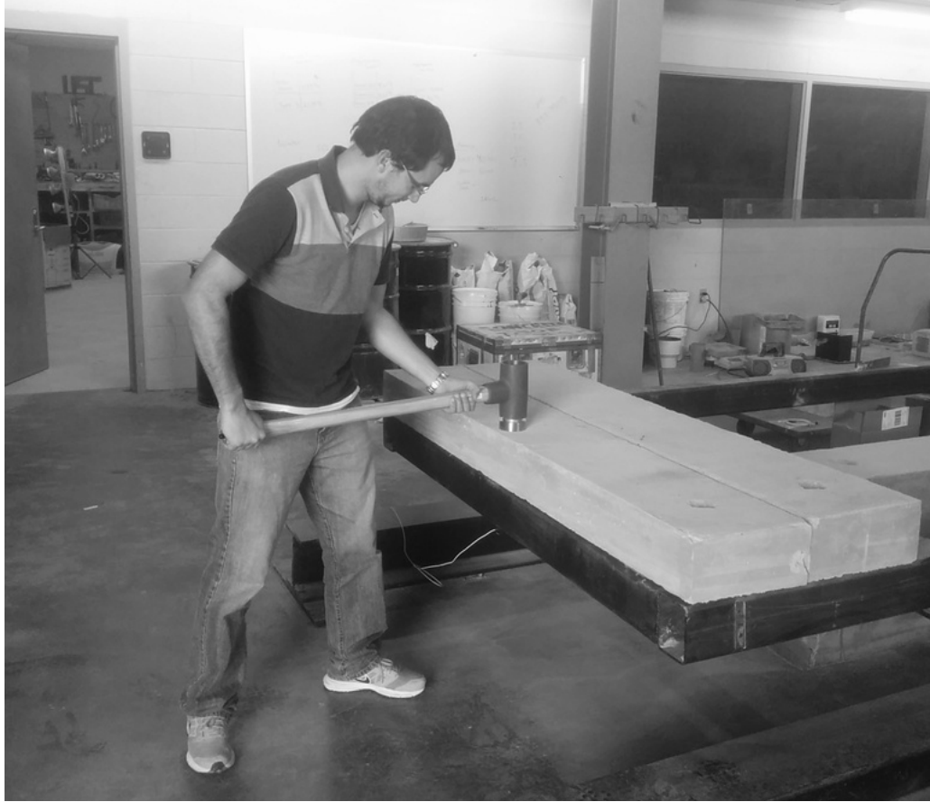
Figure 3.3: Typical free vibration test performed at the structure
