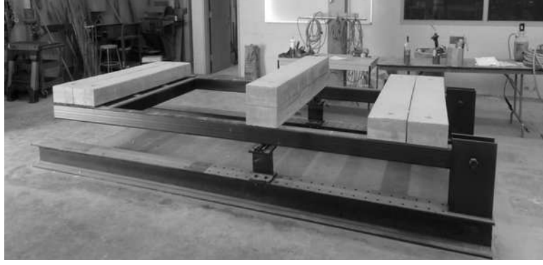
Figure 3.2: Test configurations: Empty structure
